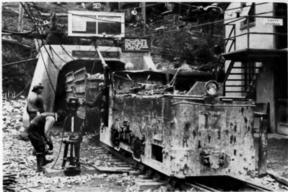
Bringing out the molybdenite ore at Climax. The mine attained a production of 20,000 tons of ore a day during the war and Climax delivered nearly 50,000,000 pounds of molybdenum to industry in the peak year of 1943. —Earth Science Staff Photo.
